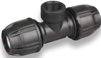
Metric Female Tee Poly x Poly x F.I. BSPT
